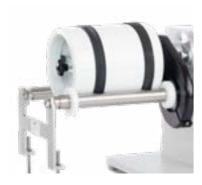
The balls are made of porcelain with a diameter from 30 to 50 mm. The drum is sealed airtight with a lid and is delivered including a frame for the drive unit. The drum and balls can be sterilized in water. For using the ball mill, a drive
