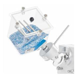
The Cube Mixer uses a tumbling motion to produce a homogenous blend within a short time. The mixing action is assisted by three stainless steel rods positioned inside the cube. The device is attached to the drive unit via the ERWEKA Universal Gear UG, which permits operation at various angles for optimal efficiency. Our cube mixers are available in the following versions:
