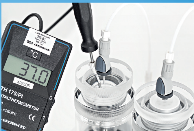
Special temperature calibration head
